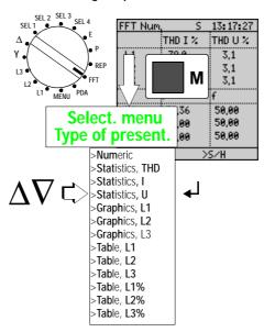
Set the *rotary switch* to the FFT position. The display shows the actual total harmonic distortion of current and voltage, the phase power and the frequency of all three phases.
